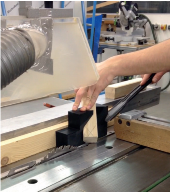
Cutting tool for the first two cuts: It is not advisable to cut on the right side of the blade
