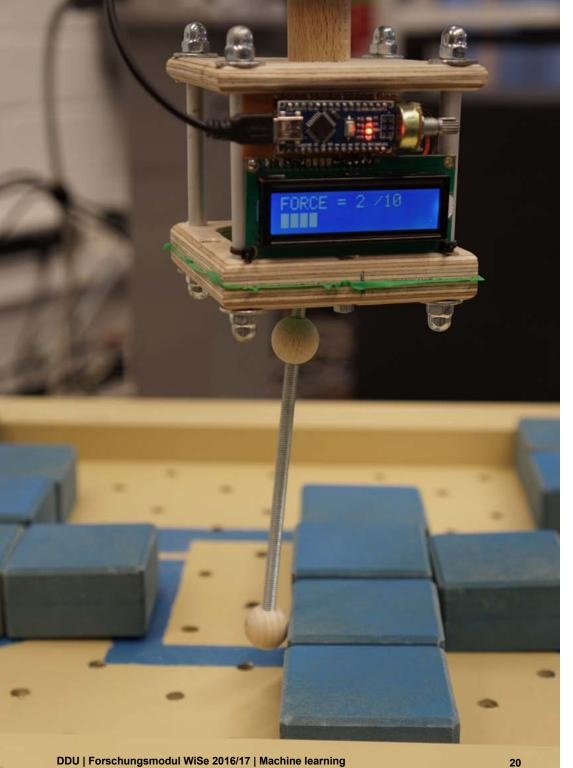
The ARDUINO checks constantly for changes in the values from the two potentiometers. If the change exceeds a certain amount, the Arduino sends an integer via USB corresponding to the deflection of the rod. If no obstacle blocks the movement, the value equals zero.
