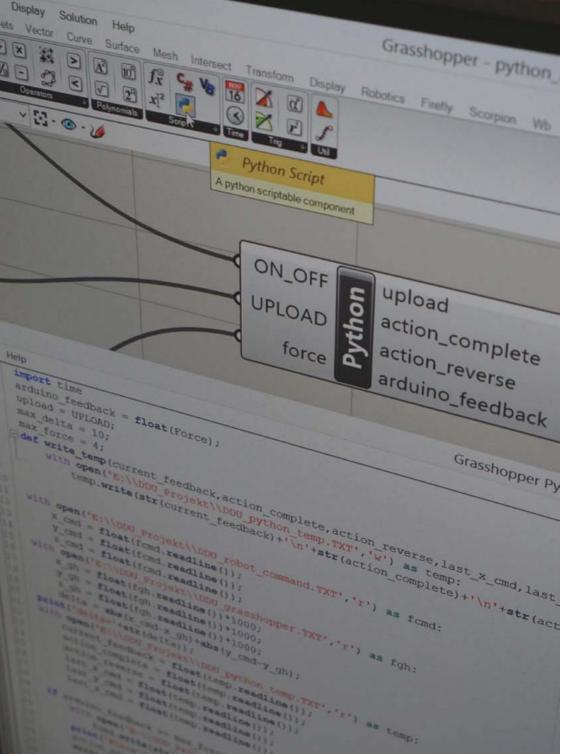
A PYTHON SKRIPT, embedded in a dedicated Grasshopper file, checks the incoming values from the serial port the Arduino writes to. Besides that, it keeps track of the difference between the actual position of the robot and its destination. They are read from the ".txt-files" Grasshopper and Matlab write into.
