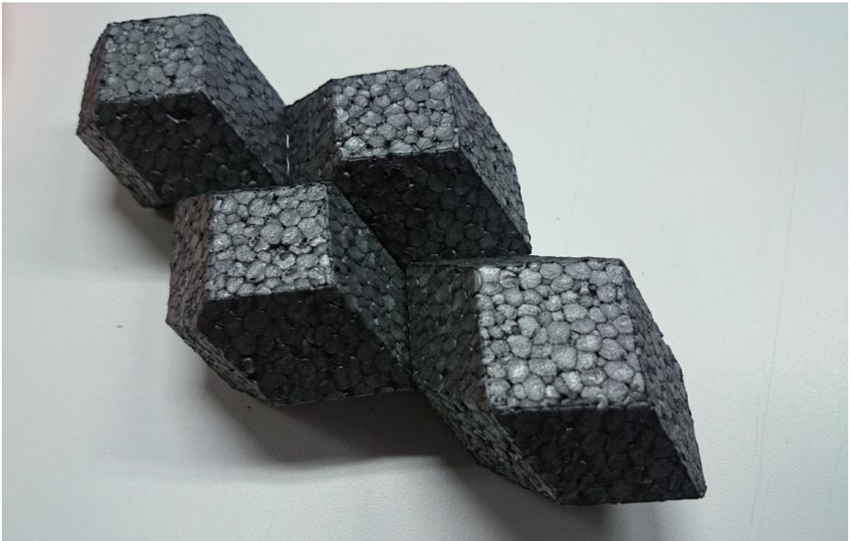
\* The test of cutting G2 in different size shows the importance of the size in CNC hotwire cutting. The bigger the figure is, the more presice you can get. When it's really small, then 1mm is almost part of your figure, and this error will make your form change.
