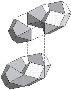
Fig. 2 The hendecahedra form interlocking hexagonal "boat" shapes.
